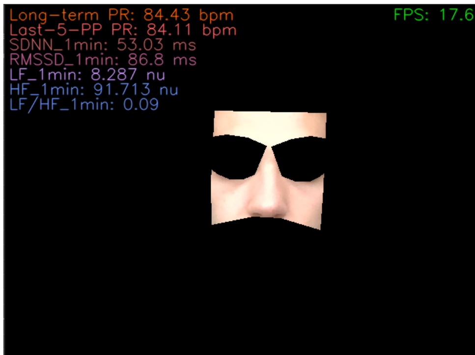
Figure 3.11: The output of the algorithm. In the top left corner, we can see both pulse rate (long-term PR and last-5-PP PR) and pulse rate variability (SDNN, RMSSD, LF, HF and LF/HF) readings.
